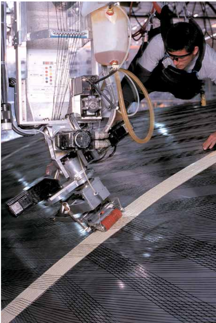
[Left] A North sailmaker applying carbon-fibre thread to a high-tech sail. [Below] A 3DL mold in North Sails' plant in Minden, Germany.
