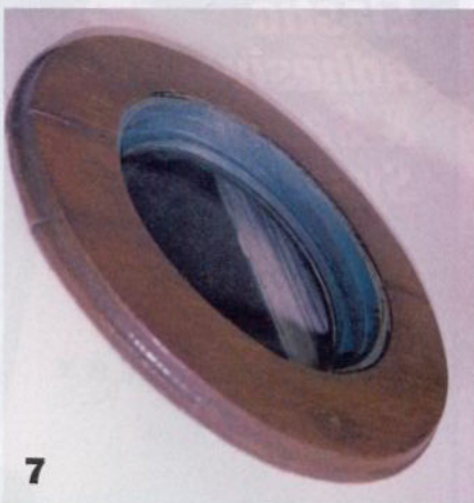
7 With the wooden trim ring back in place, the porthole is watertight once again.
