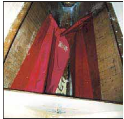
(left) Measuring fiberglass to cover the engine beds. (right) Applying peel ply to the fiberglass to leave a smooth appearance.
