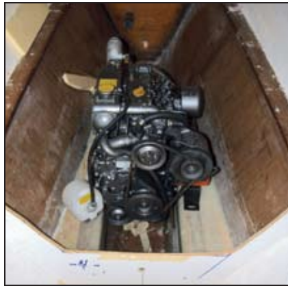
(left) There wasn't enough height over the engine for a block and tackle, so a lifting rope was lead through a block to a winch outside on deck. The overhead lifting beam was suitably braced. (right) Engine on the beds.
